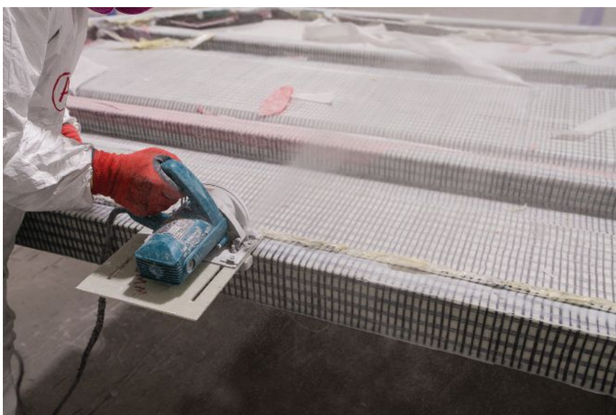
■ Ceiling panels such as these (shown shortly after demolding at top and during trimming at bottom, before any insulation layers or exterior elements were added) incorporated hybrid glass/carbon fiber fabrics laid up with epoxy over structural foam core, reinforced with foam or composite stringers.
