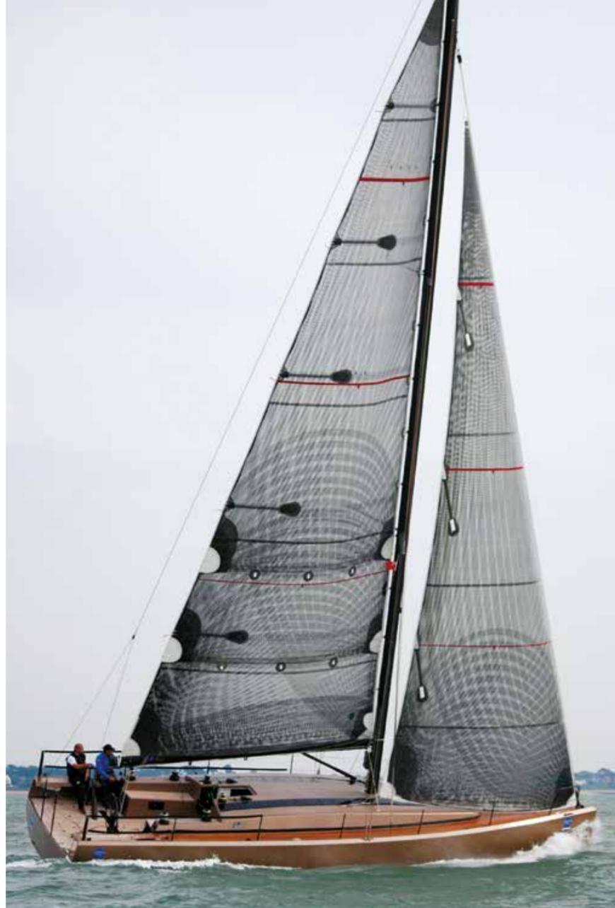
The first boat is fully loaded (to the point that the final cost is a source of some embarrassment), with all main Harken primary and pit winches powered. The short headsail tracks are on a manual pin system, simply to keep the decks free of rope work. The backstay, vang and outhaul are all hydraulically controlled on this boat.
